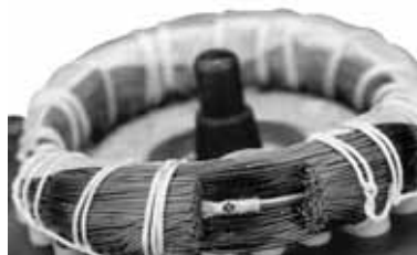
Fig. 28 PTC sensor incorporated in windings
