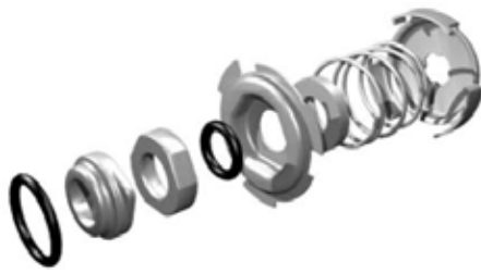
Fig. 10 Exploded view of shaft seal
