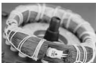
Fig. 30 Thermal switch incorporated in windings
